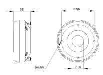
220 W continuous program power capacity 1.4" horn throat diameter 75 mm (3 in) aluminium voice coil Titanium diaphragm 500 - 18000 Hz response 108 dB sensitivity
